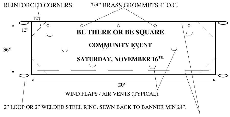
MIN 1" MAX 1 ½" NYLON WEBBING ENCASED IN SEWN SLEEVE, TOP & BOTTOM, ENTIRE LENGTH OF EACH.
