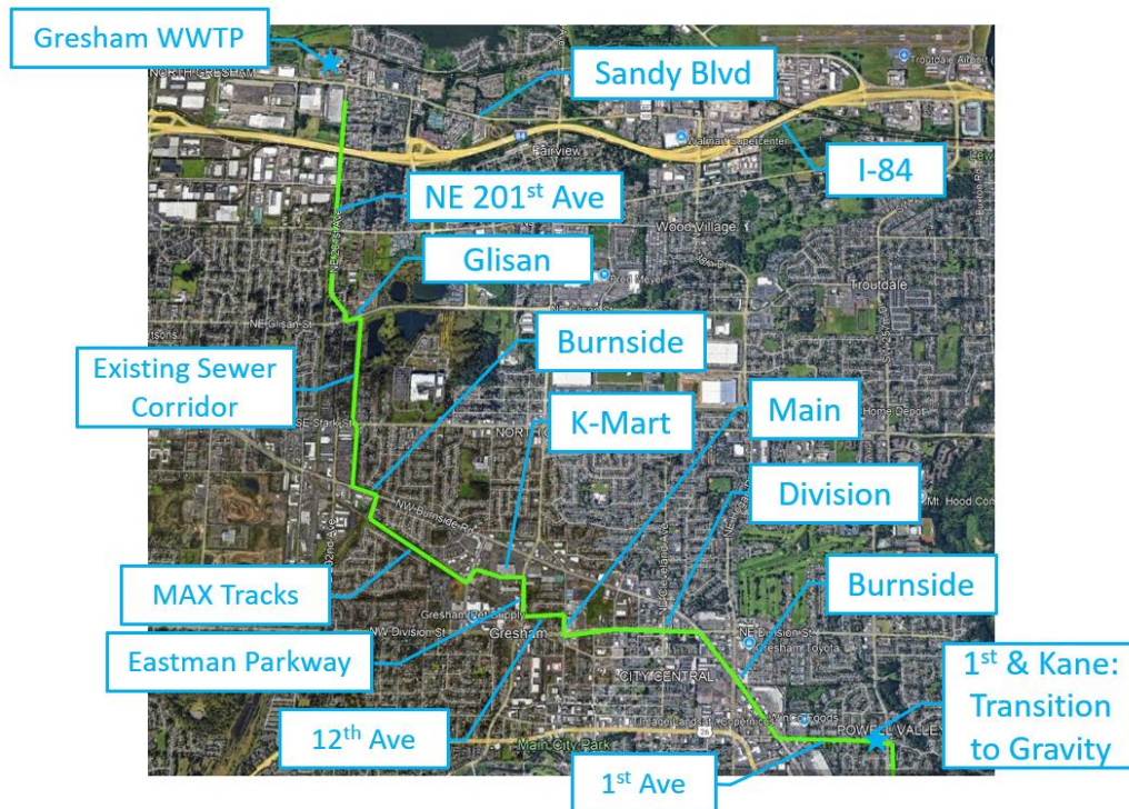
Figure 2. Alternative 1 Gravity Main Alignment
