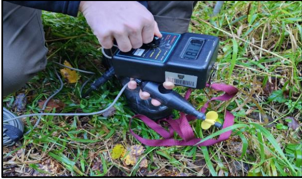
Image 9: Swiffer Flow Meter – Calibration and Setup
