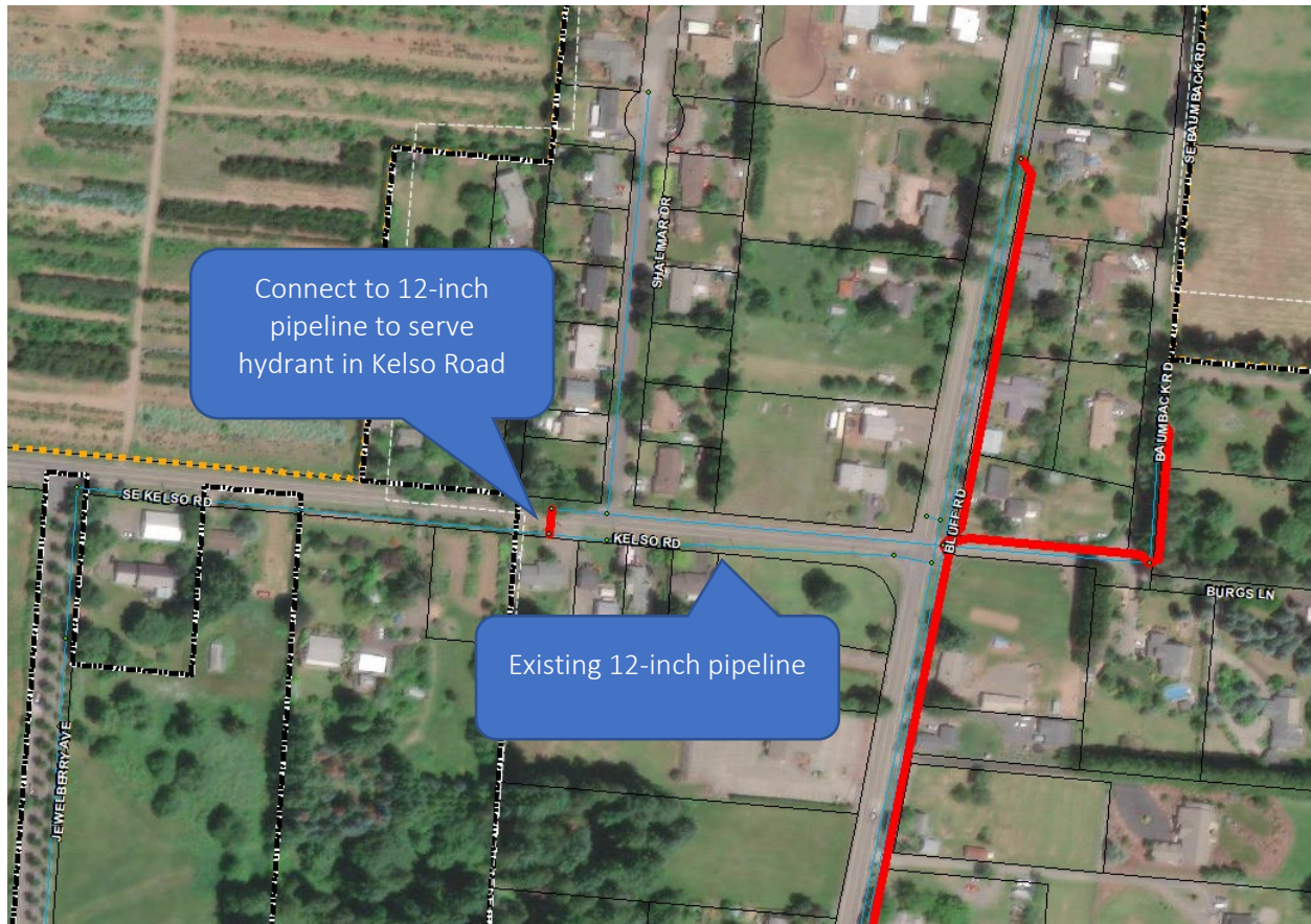
Figure 4-12 | Kelso Road Improvements
