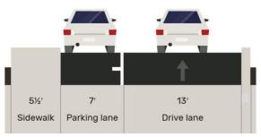
FIGURE 11: JUNKER STREET CROSS-SECTION WITH PARKING
