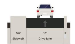
FIGURE 10: JUNKER STREET CROSS-SECTION WITH EXISTING RIGHT-OF-WAY
