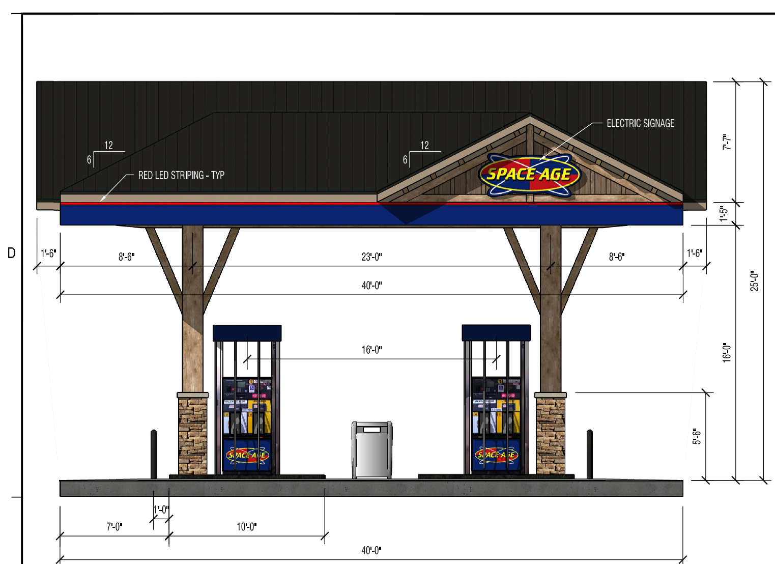
C1 NORTH AND SOUTH ELEVATION 3/16"=1'-0"
