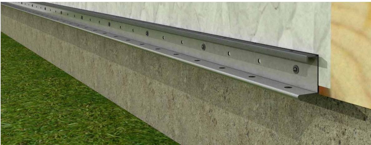
Vertical Starter Track fastened every 6" to 9" to framing.
