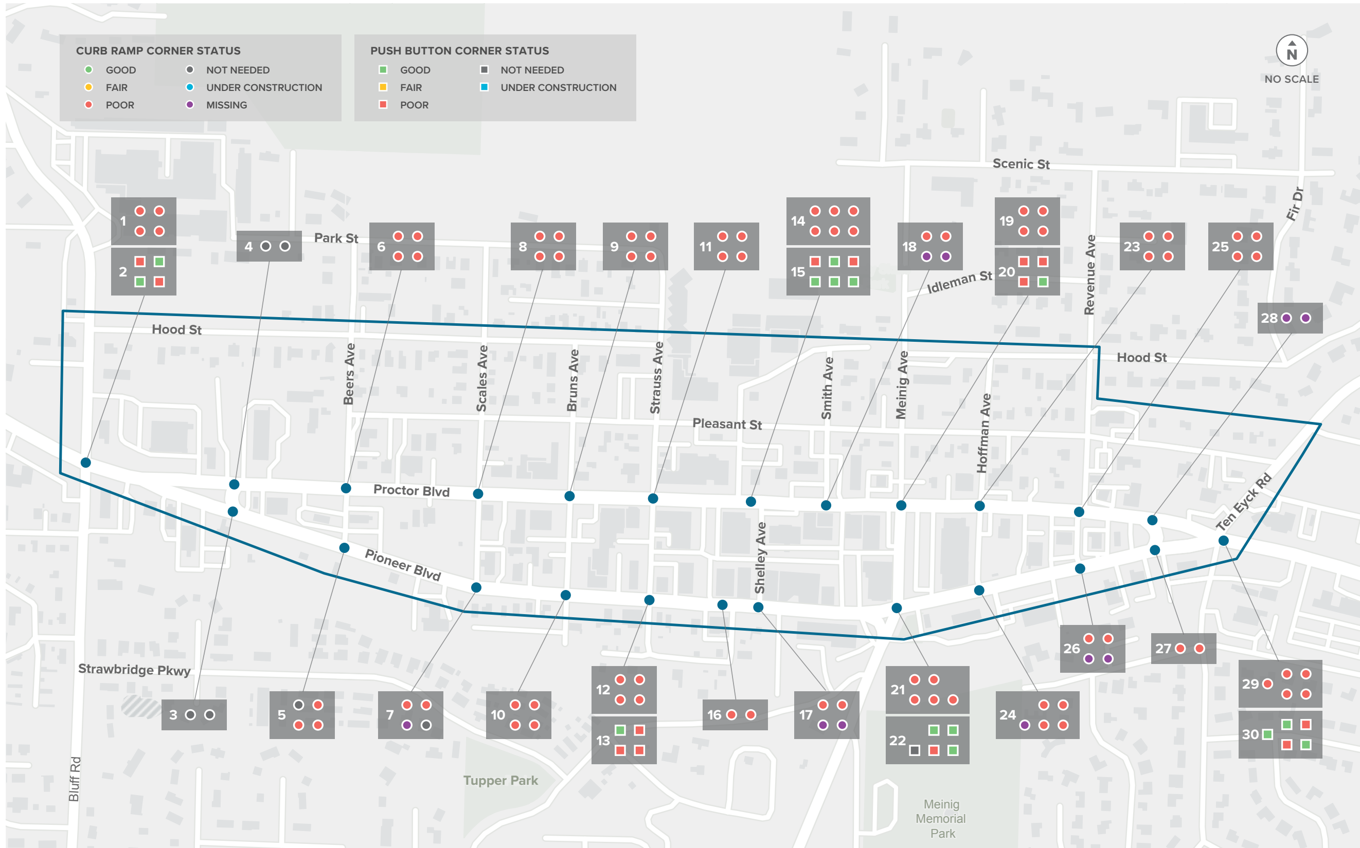
FIGURE 7. CURB RAMP AND PUSH BUTTON ACCESSIBILITY CONDITIONS
