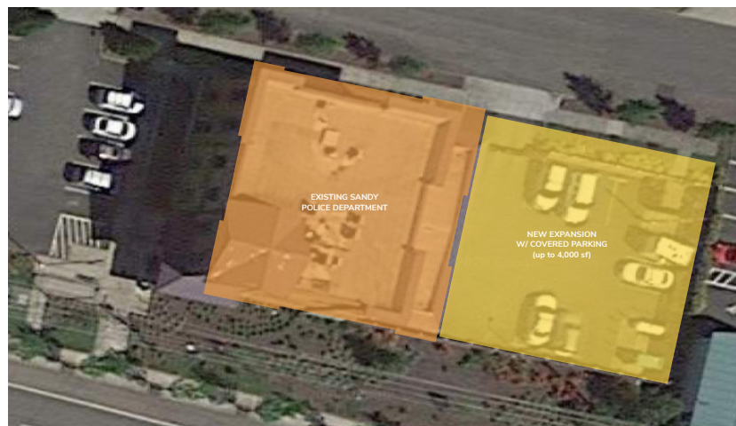
An example of design Option 2, the existing building is expanded to the east with covered parking on the ground floor.
