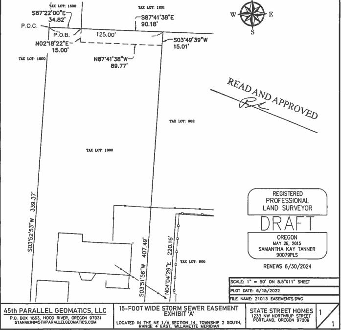
BASIS OF BEARING IS PER GPS OBSERVATION ON CONTROL POINTS.
