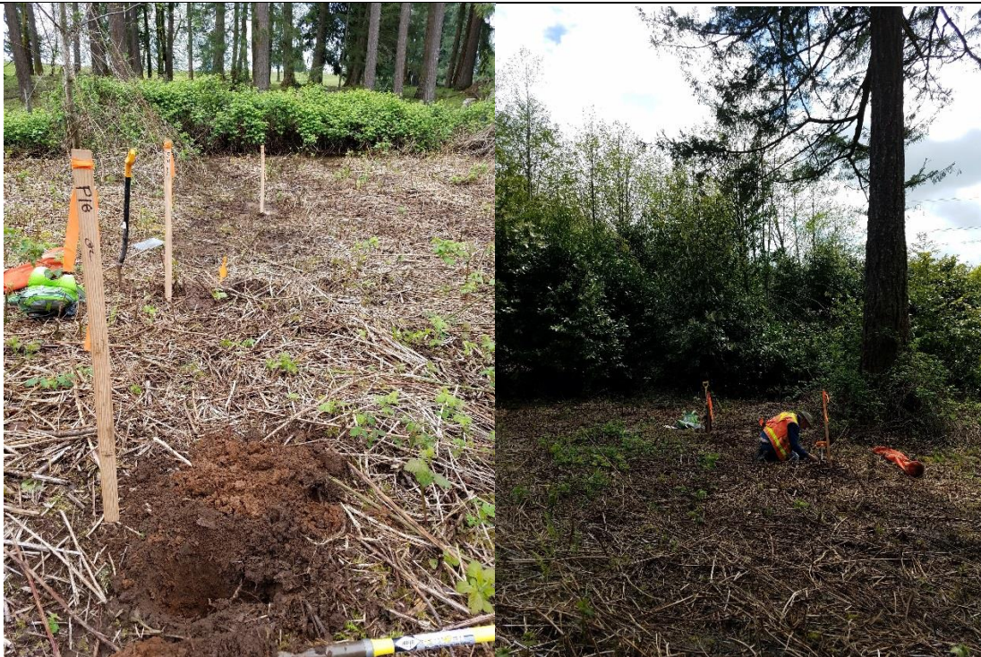
Photo 4, (left) and 5 (right). Wetland "C". Photo 4 looks down toward the stream, and 5 looks up from the stream. P18 had dry non-hydric soils, and saturated hydric soils were found at P17 which is slightly lower and closer to the stream.
